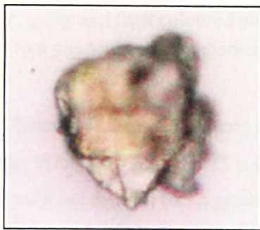
Figure 57. Shell white (X 400 Magnification). Chinese Drawings of Plants Small Volume II. (The Royal Horticultural Society)
