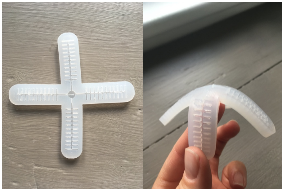
Figures 20 and 21: Testing of curing silicone in moulds
