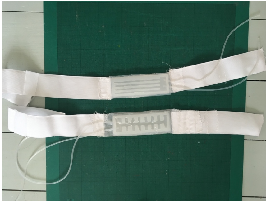
Figure 22: Testing different shape inflatables and attachments
